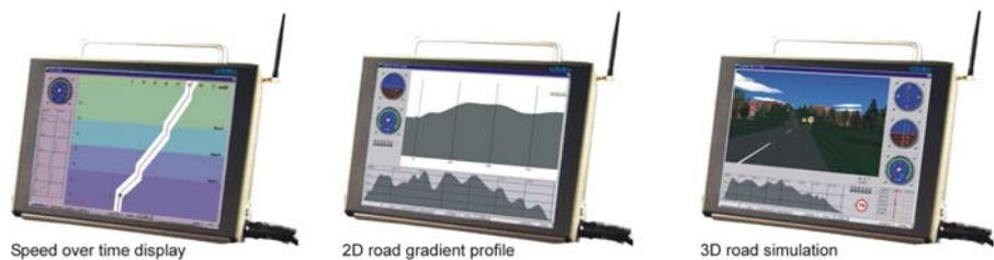
Figure 1: Illustration of the three main modes that are a part of the ErgoDrive Professional system
